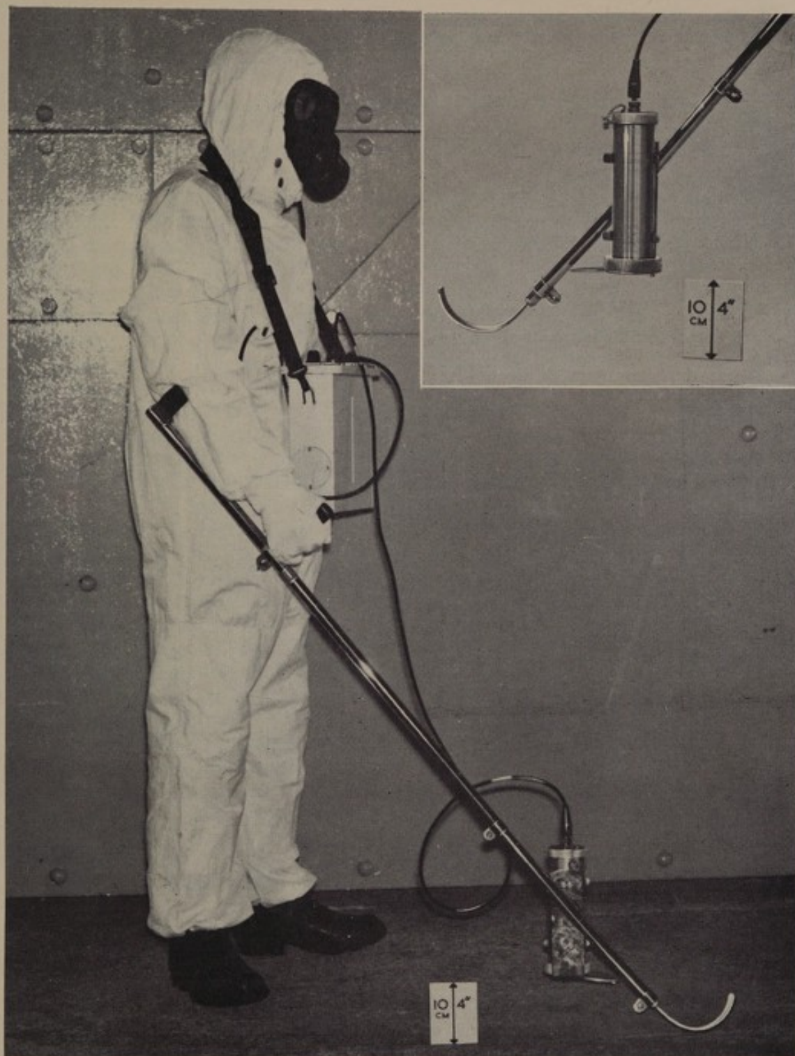
FIG. 2(R). THE 1320 MONITOR WITH ALPHA DETECTOR IN OPERATION In the field the whole assembly would be polythened as a protection against contamination. The insert indicates the ground to probe-face distance.
