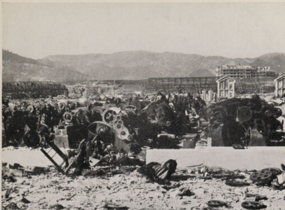
Photo No. 13. NAGASAKI. \frac{1}{2} mile from centre of damage. Typical damaged machines in one of the many timber workshops destroyed by blast and fire. Some machines were overturned by movement of the buildings, some destroyed by fire alone ; others damaged by exposure to the weather. See paragraph 34.
