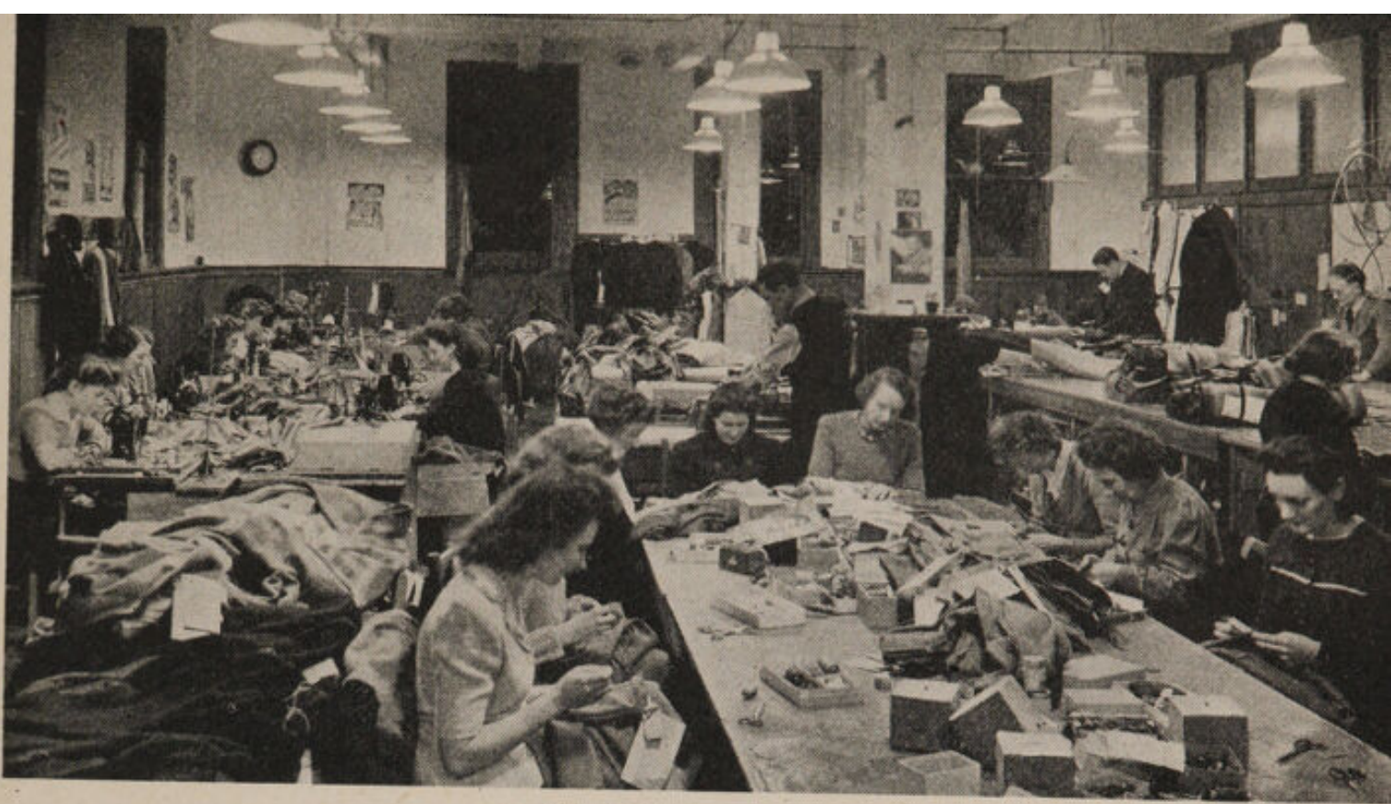
Fig. 23. Sewing without eye-strain and without mistakes under 18 foot-candles of diffused lighting. The higher glass brightness of these 200-watt glass-steel fittings is acceptable, because the glass is screened by the reflector. Photo: Forward Fashions, Melbourne, Vic.
