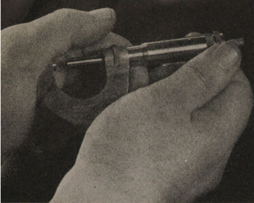
Fig. 7. Reflected glare makes this micrometer scale very difficult to read. Scales on polished surfaces require well-diffused lighting.
