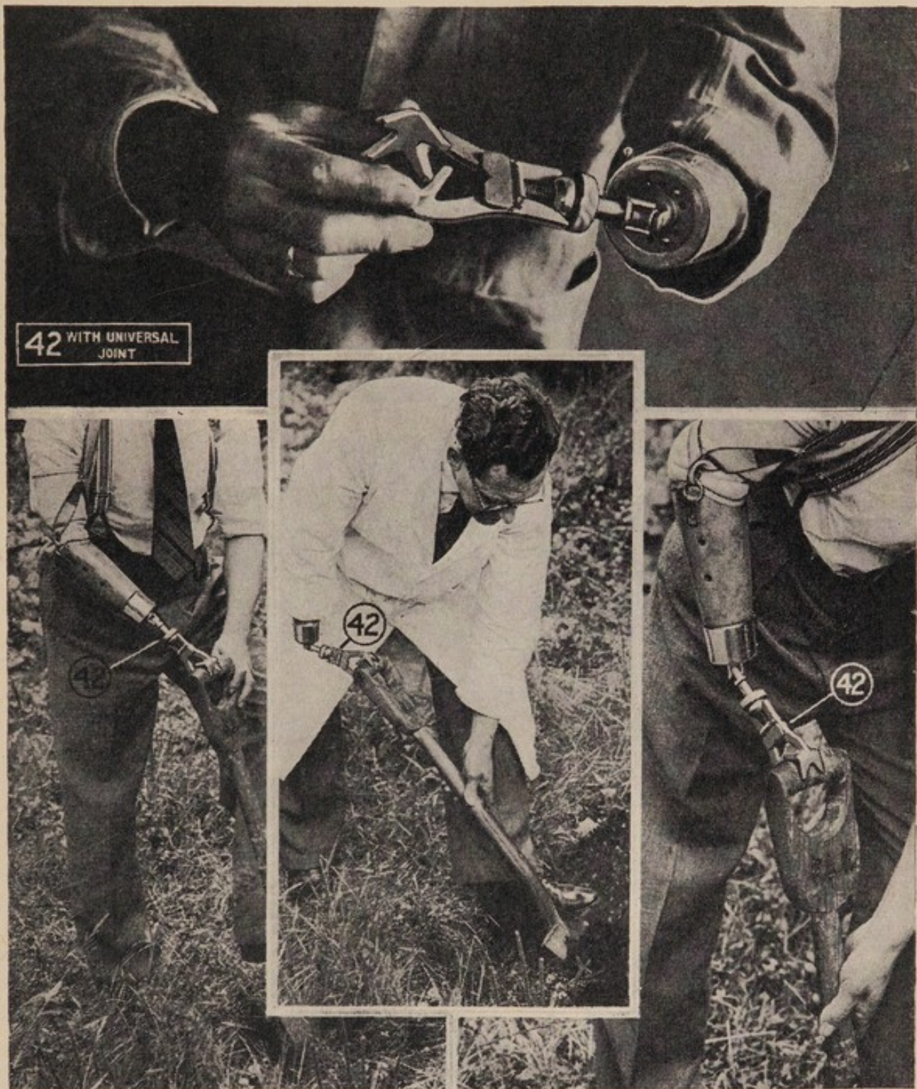
Artificial Arm Appliance. The Tool and Implement Holder in use. Reprinted from Production and Engineering Bulletin.
