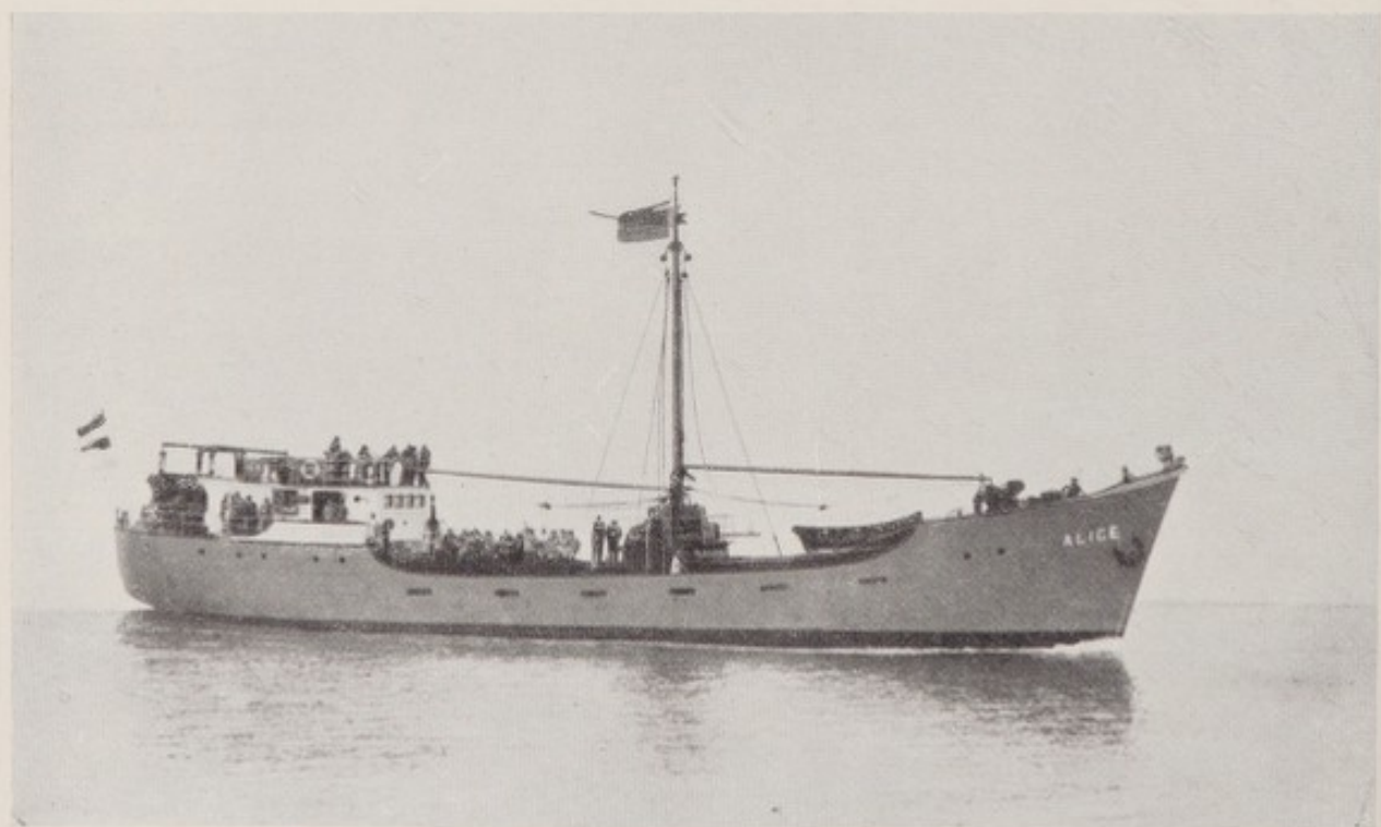
Plate 40. The Alice , a modern Dutch motor coaster This vessel, with a length of 127 ft. and a beam of 23½ ft., has a gross tonnage of 291, and a net tonnage of 320. She was built in 1939 by Van der Werff Scheeps. at Westerbroek near Groningen , and was engined by Appingedammer Brons Motorenfabriek , Appingedam.
