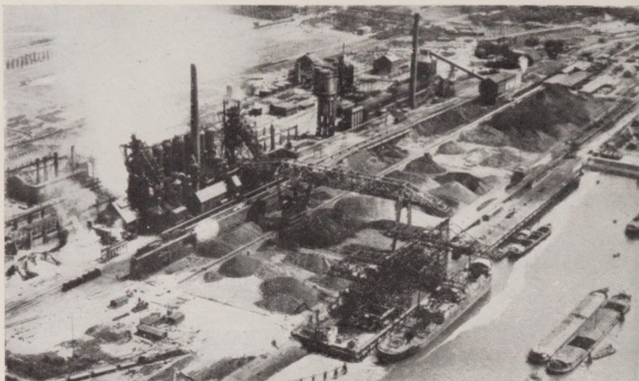
Plate 55. Ymuiden : Hoogovenhaven and steel works, looking north-east This is one of the largest steel works in Europe, operating three blast furnaces, coke ovens, chemical works, cement works and steel mills.
