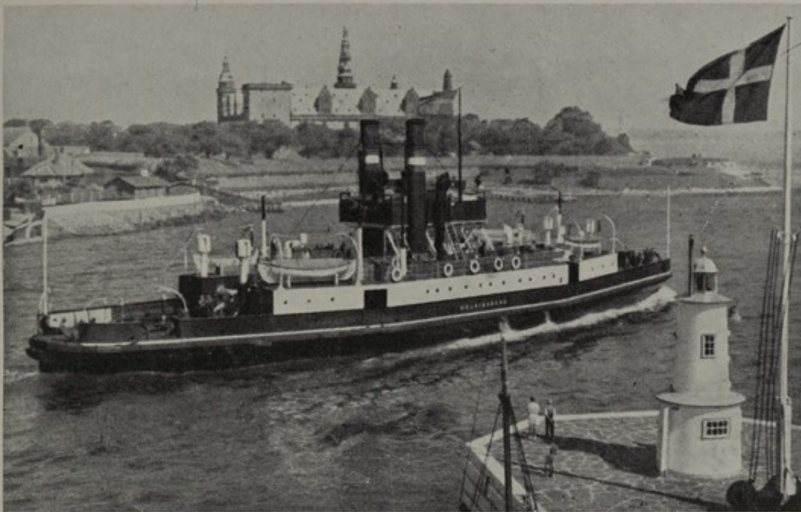
Plate 97. The train-ferry Helsingborg entering Helsingør (Elsinore) harbour The ship is of 530 gross tons and has one rail track. She is used for both the train and car ferry services between Helsingør and Hålsingborg.
