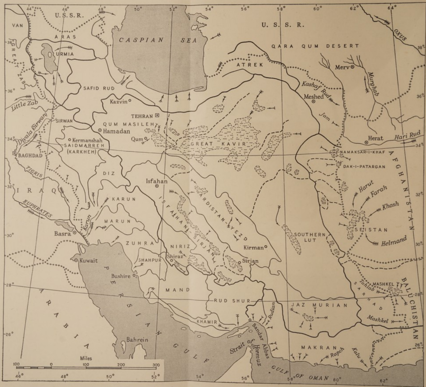
FIG. 8. Drainage basins of Persia. Primary watersheds are shown by thick lines; less important watersheds by thin or broken lines. The relative importance of river discharge is shown by the number of 'feathers' on each arrow.
