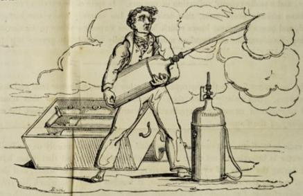
When a small quanty of simple water is cast on materials in a state of VIOLENT combustion, it evaporates into steam from the heat, the addition of other fixed incombustible ingredients consequently becomes necessary, to make quality supply the place of quantity.
