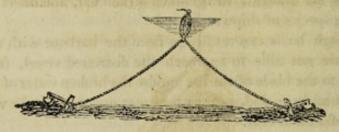
yards from each other, are to be laid out parallel with the shore, some distance beyond the point at which the waves break in surf. These are to be connected by about forty fathoms of strong rope or hawser, the slack of which is to be suspended by a buoy fixed on the centre, as in the plate.
