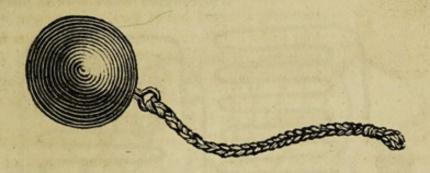
The hide should be at least so long as to leave two feet beyond the muzzle of the mortar when it is charged with the shot, and should have a loop at its end, that the rope may be fixed to it in a moment. The strips of hide may also be braided in the manner used in making the thongs of whips.
