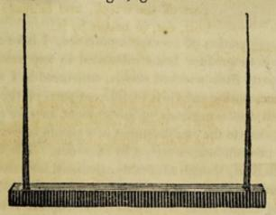
afforded leisure to place a frame (like the figure) in exact line with the vessel, by which the aim of the mortar is then to be directed. This frame is made of a piece of wood 4 feet long, 9 inches wide, and 3 inches deep, (so heavy as to give a requisite degree of steadiness from its own
