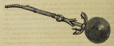
This shot is to be used, when the crews of the distressed vessels, from exhaustion by fatigue, numbness from cold, or from having previously lashed themselves in the rigging to secure themselves from being swept away by the sea, which breaks over the vessel, are deprived of the power of assisting themselves in the slightest degree. The advantage gained by the use of this shot is, that, when the people on the shore haul in the rope which it has carried over the vessel, it catches
