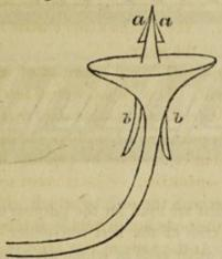
a a are barbs fitting with springs into mortices on the sides of the point.
