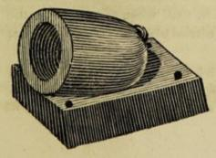
The mortars, for the purpose of throwing the shot with the line attached to it, over the wrecked vessel, should be as light as is compatible with the service to be performed by them. An iron mortar\* cast on its bed, and weighing with its bed 2½ cwt. (which may be removed from place to place by two men on a hand-barrow with ease) will project a 24 lb. shot, with an inch and half rope attached to it, 250 yards, or a deep-sea line 320 yards, against the utmost power of the wind.
