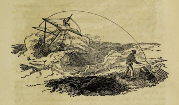
When the rope is thrown on board, the crew, if not extremely exhausted, will at once secure it to some firm part of the wreck, and then a boat\* (if a boat be at hand) may be hauled off by it: the boat is kept, by the power given over it by the rope, with its head to the waves and wind; and consequently rises over the surges, free from the danger of being upset.
