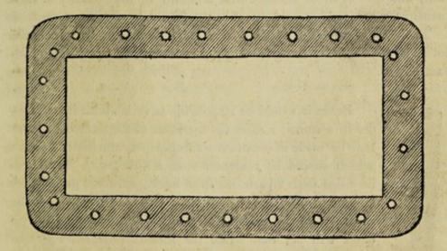
These pegs should be of an inch and a half diameter at the base.
