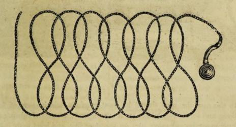
It is however necessary to observe, that the greatest attention and caution are required in laying the rope in conformity to the two latter methods. They are more complex, more easily deranged by the wind (which, from the fakes being raised on each other, is admitted under and lifts them) or other accidents, and any derangement not so easily detected by the eye as in the first method proposed, nor when detected so instantaneously rectified.
