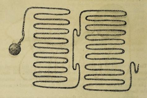
The length of the fakes must not exceed two yards, as the rope, when laid in fakes of greater length, is likely to be broken by the proportionably increased vibration. When the experiment was made with the rope laid in fakes of several yards long, it never failed to break.
