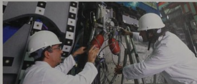
▲ Setup of a large-scale structural test (industrial building shear-wall) at the European Laboratory for Structural Assessment (ELSA) Laboratory: Hydraulic high-pressure hose connection to the actuator's servo-valve.
