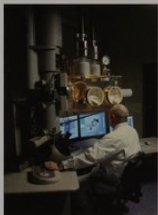
New transmission electron microscope, installed at the JRC-ITU for the analysis of radioactive materials.
