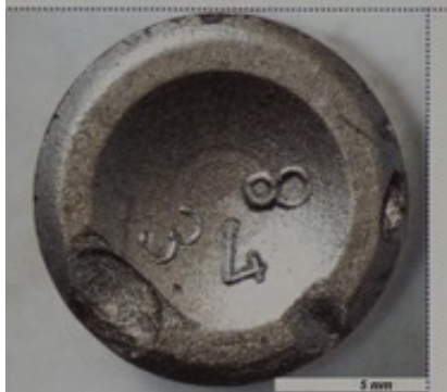
One of the uranium fuel pellets seized in Lauenförde (Germany). The pellet shows mechanical defects and markings on the top and on the bottom
