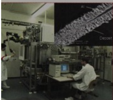
Pilot facility for pyrometallurgical reprocessing as developed at the JRC-ITU. The inset shows a Scanning Electron Microscopy image of the cross-section of an Al electrode which has a An loading of 59.9 wt. %
