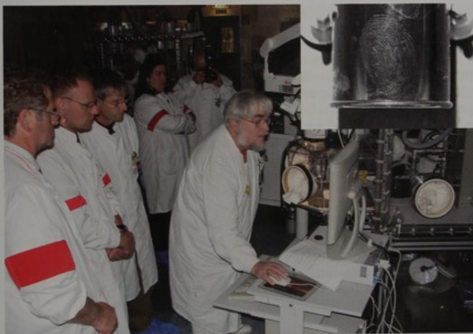
BKA ("BundesKriminalAmt") delegation being shown the operation of a glove-box for the implementation of classical forensic methods on contaminated materials developed in collaboration with JRC-ITU. The inset shows a digital print on a radioactively contaminated material.
