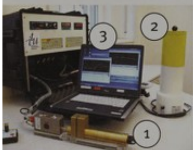
Photograph of the COMPUCEA 2 nd generation with L-edge spectrometer (1), \text{LaBr}_3(\text{Ce}) detector (2), data acquisition hardware (3) and PC. The equipment is small enough to fit into a suitcase
