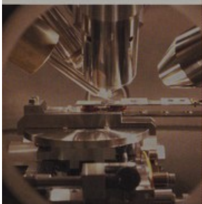
TOF-SIMS (Time of Flight - Secondary Ion Mass Spectrometry) chamber detail of bar for multi sample analysis
