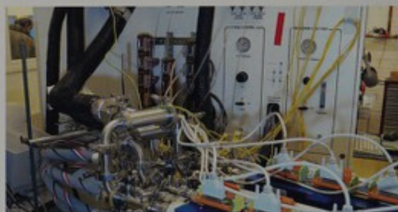
Fuel cell stack undergoing testing in the Petten facility
