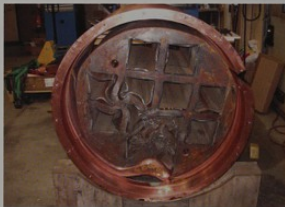
Mock-up after plastic collapse at pressure load of 139 MPa
