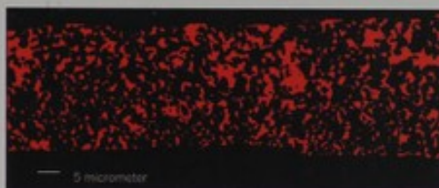
Digital, 2D image of the pore matrix. Pores are depicted in red
