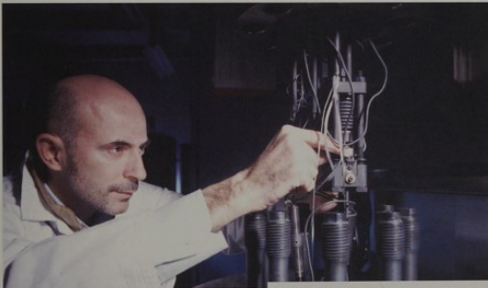
Loading samples in the special autoclave designed to test stress corrosion cracking
