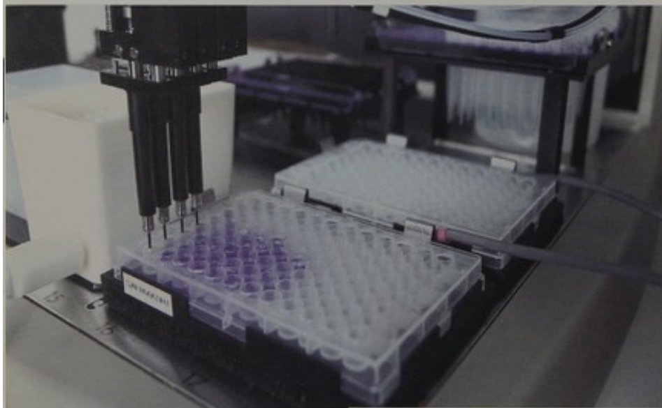
Automatic protein digestion and sample preparation for mass spectrometry
