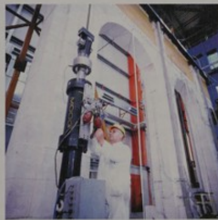
S. Vicente test model at ELSA. Servo-actuator for vertical loading.
