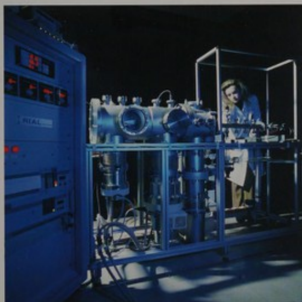
Chemical ionisation mass spectrometer (CIMS) with flow tube reactor for studies of atmospheric chemistry.
