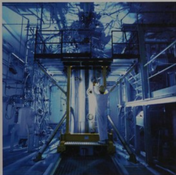
FAT (Faro Advanced Tank) vessel for molten fuel/coolant interaction
