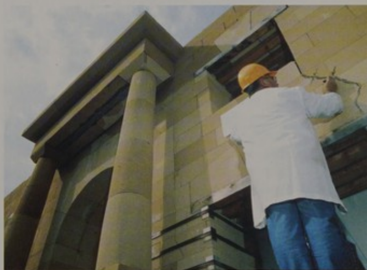
Palazzo Geraci facade model post-test identification of the damage zones (cracks).
