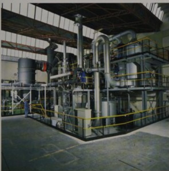
Small incineration plant for the investigation of advanced waste treatment processes.
