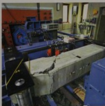
Dynamic testing on a reinforced concrete beam in the Large Dynamic Test Facility (LDTF).
