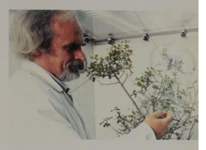
BEMA Project: study of biogenic emissions from a Mediterranean oak using a Teflon® cuvette in the environmental chamber (phytotron)
