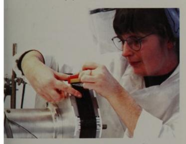
Fabrication of preforms for fibre-reinforced ceramic-matrix composites
