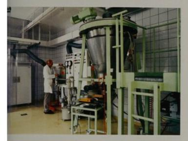
Installation for grinding, mixing and sampling to be used for the preparation of high quality reference materials
