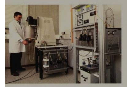
Facility for thermogravimety with gas mixing and analysis station for high temperature corrosion testing up to 1700° C
