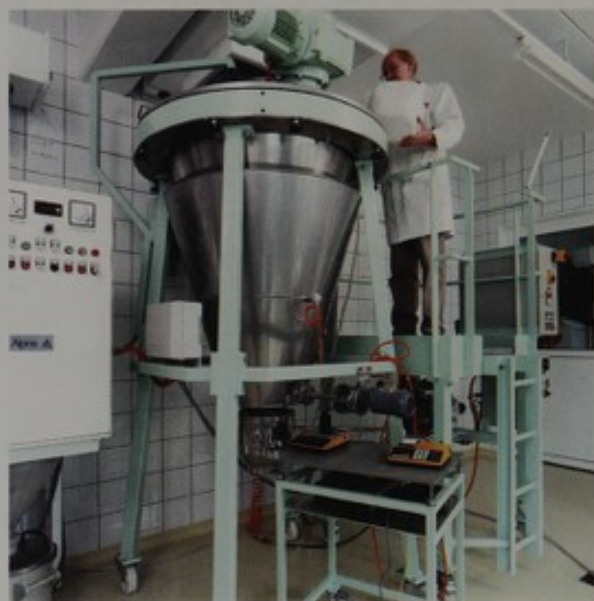
Multipurpose mixer with filling equipment. Heat treatment and homogenisation of large amounts (up to 200 kg) of soils and sediments. Filling bottles with well homogeneous powders.
