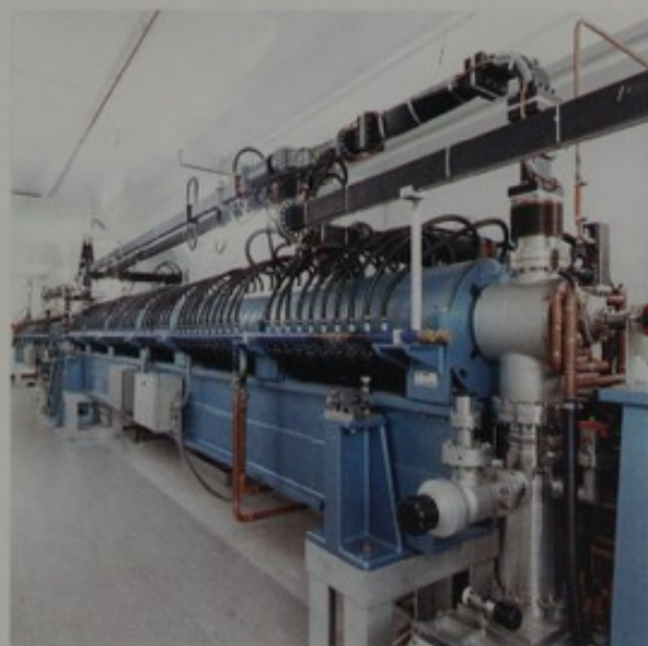
The refurbished LINAC; view of the new accelerating sections.
