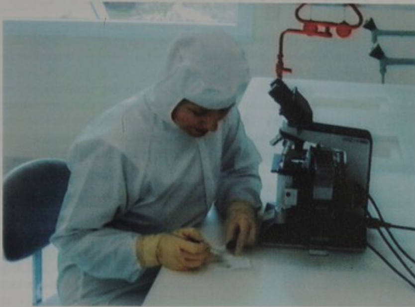
Preparation of specimens in the 100 class clean laboratory ARTINA for the analysis of particles in swipe samples.
