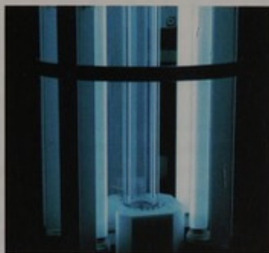
Partial view of the vertical laminar flow reactor (bottom). Facility to study the formation and the properties of submicron aerosol particles.
