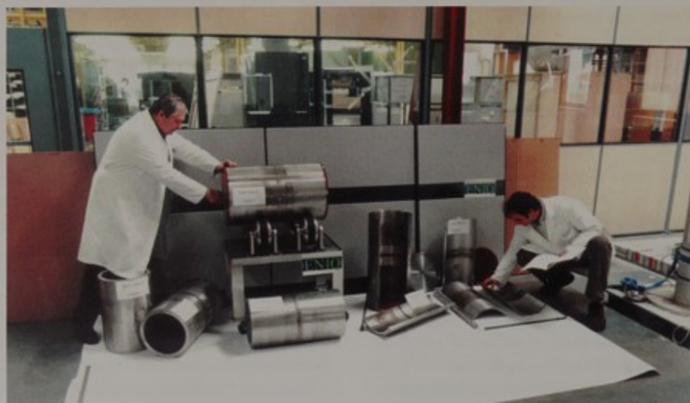
Test assemblies used for the pilot study on the application of the European Methodology for Qualification of inspection procedures.
