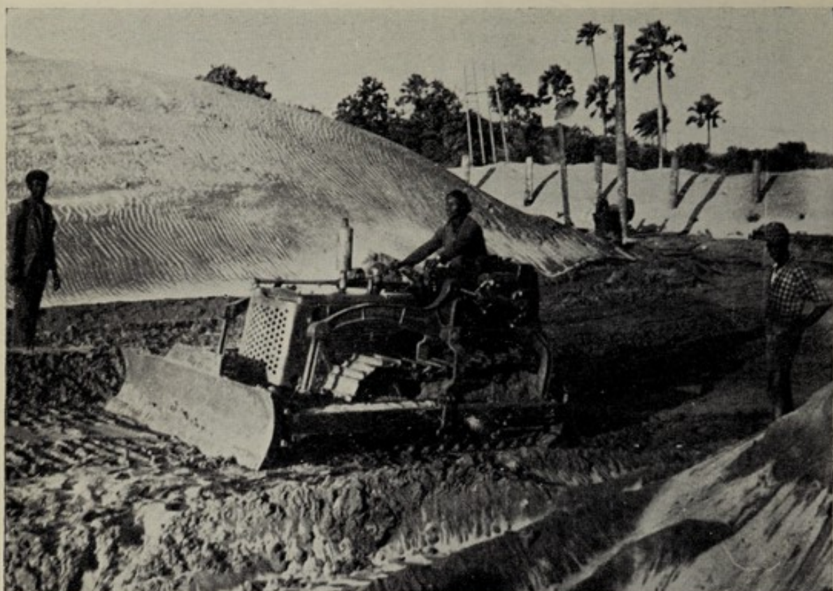
Piling heavy mineral concentrate by bulldozer at the Gambia Minerals, Ltd. site at Brufut.
