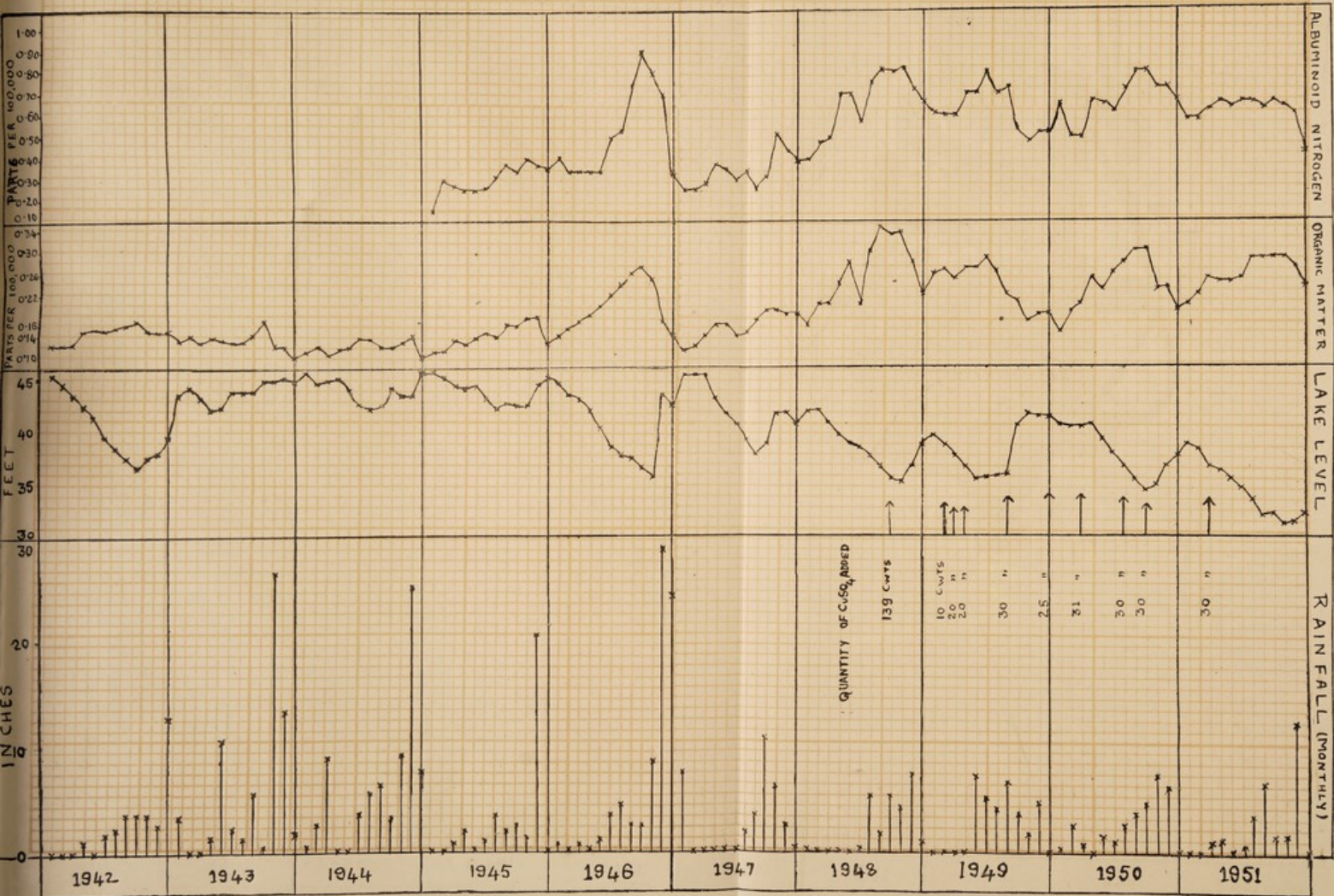
Madras City - Graph II Relation between Rainfall, Lake Level, Oxidisable Organic matter (Tidy's) and Albuminoid Nitrogen for 1942 - 1951
