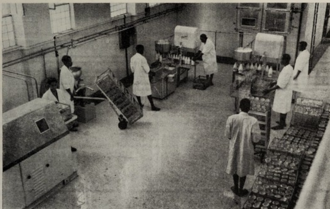
A portion of the new Oriental Dairy showing the "IN-CRATE" bottle washer, bottle filler and cabinet cooler.
