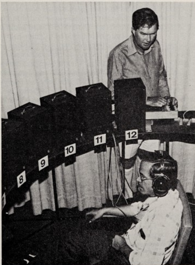
The directional hearing of a patient is measured with earphones mounted on earmuffs by audiologist Mr Denis Byrne, of the Audiology Services Section of the National Acoustic Laboratories central laboratory in Sydney.
