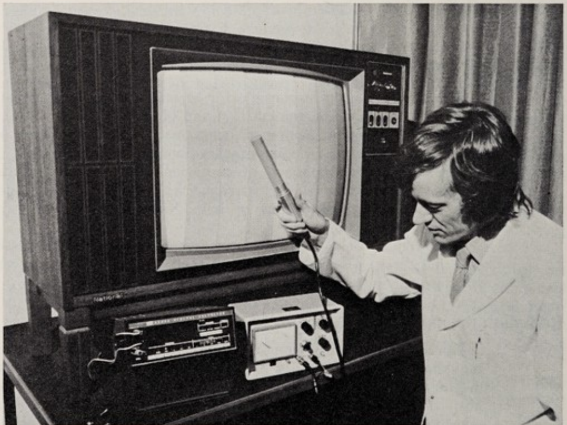
Mr Peter Burns, a physicist at the Australian Radiation Laboratory, monitors a prototype domestic color television receiver to check X-ray emissions. Such measurements are made under normal conditions as well as under induced fault conditions which could give rise to increased emissions.
