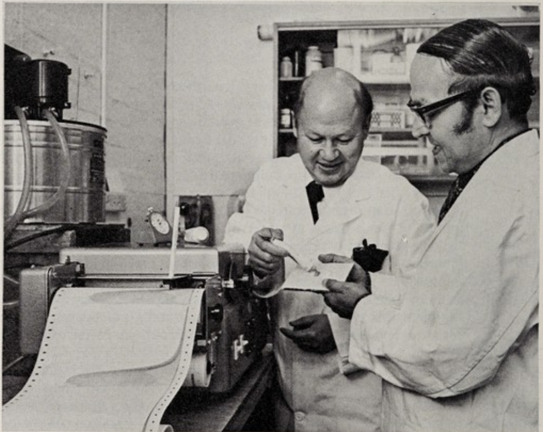
Mr Max Chong, Senior Technical Officer at the Australian Dental Standards Laboratory (left), and Mr Frank Thomaz, Dental Technician, prepare a sample of a dental impression material to test the rate of hardening.
