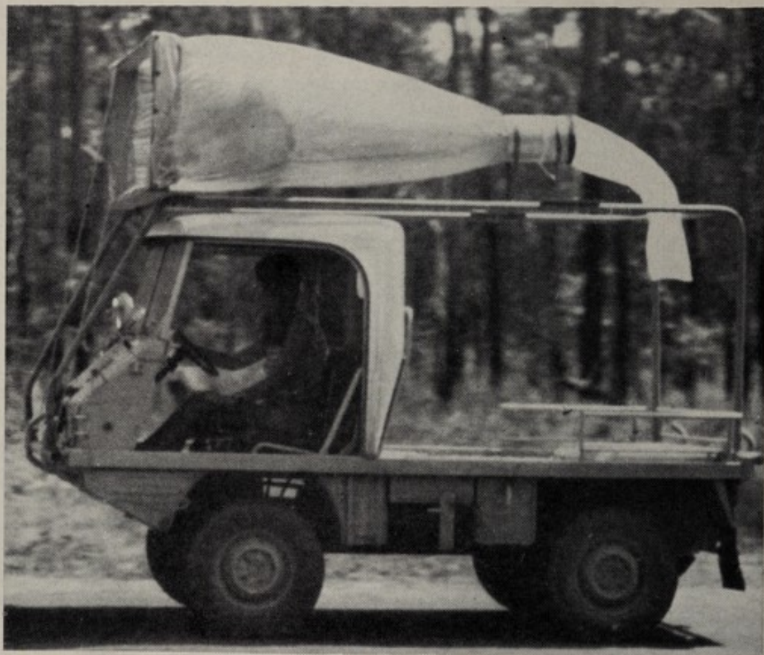
A truck trap, used by entomologists of the School of Public Health and Tropical Medicine to trap mosquitos and biting midges at Gove, in the Northern Territory.
