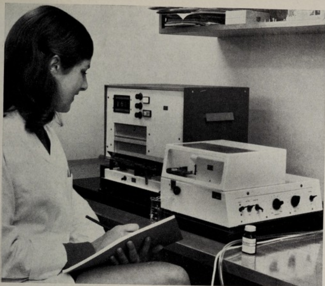
Modern automated instruments in the pharmaceutical chemistry section of the National Biological Standards Laboratory in Canberra. Above, a tablet weighing machine which is interfaced with a computer and print-out facility. It automatically determines the average weight of tablets, and compliance with official requirements. Below, a particulate matter counter which measures the number and size of foreign particles in injections.
