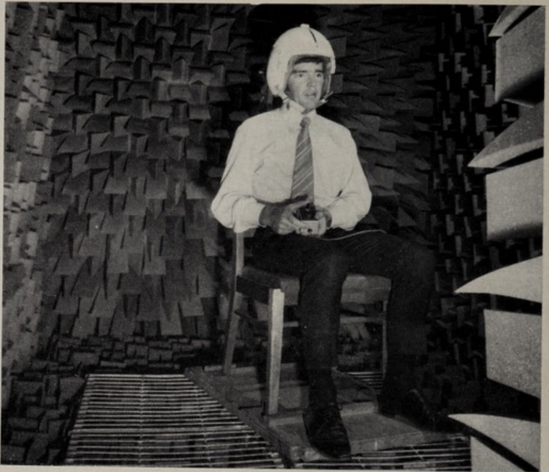
A Commonwealth Acoustic Laboratories engineer evaluating the acoustical performance of a helmet used by service helicopter crews. The test is carried out in a specially designed anechoic chamber.
