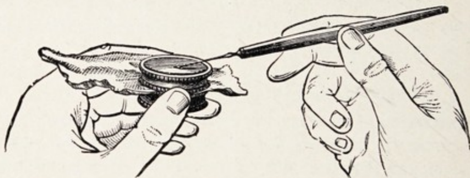
FIG. 333.—DRUM USED TO TEST THE CUTTING-EDGES OF EYE INSTRUMENTS.
