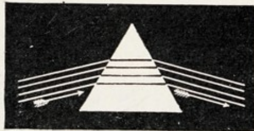
FIG. 236.—PASSAGE OF PARALLEL RAYS THROUGH A PRISM.
