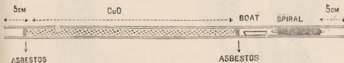
FIG. 9.—Arrangement of tube for the estimation of carbon and hydrogen.
