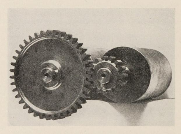
Fig. 14. Break rolls. The large and small cog-wheels are the simplest device used to give the two rolls different speeds. The larger cog-wheel is driven by power and drives the smaller, of course at a much higher rate of revolution
