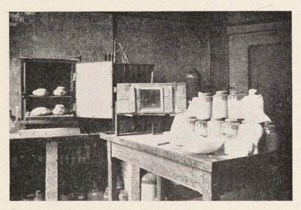
Fig. 17. The loaves shown in the last figure have just been baked and are ready to be taken out of the oven, the door of which is open. Note the different shapes. That on the right hand is obviously shown by the test to be made from a strong flour, the other from a very weak flour
