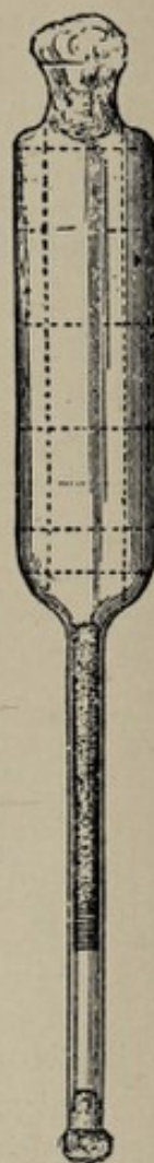
Fig. 51.—Sedgwick's expanded tube for air-examination.
