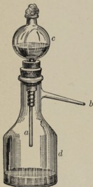
Fig. 16.—Kitasato's filter: a , Porcelain bougie; b , attachment for suction pump; c , reservoir; d , sterile receiver.
