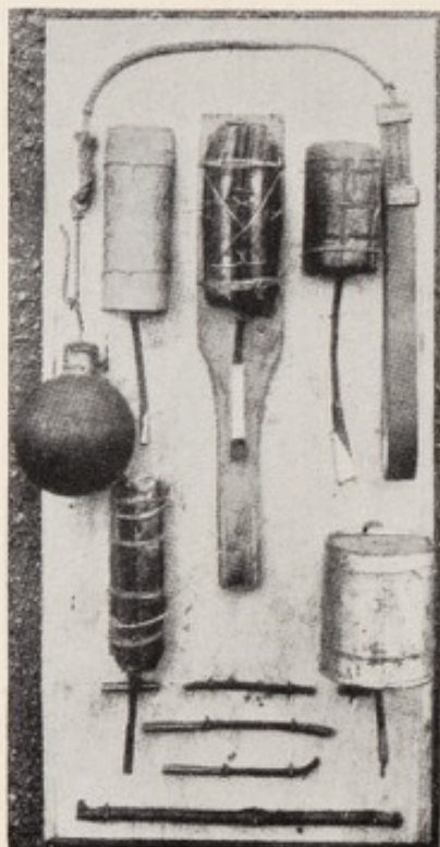
Fig. 18.—Showing the regulation French bracelet type of hand grenade and a number of ex-temporized types, such as the "racquet" and "jam-tin." (See page 14.)
