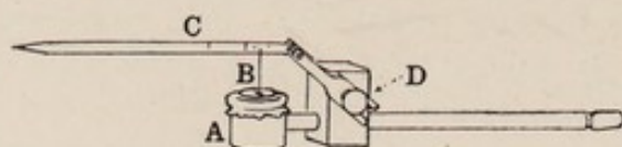
Fig. 28. Recording tambour. A, tambour; B, aluminum plate, with bell-and-socket joint for pin acting on lever; C, lever with celluloid writing point; D, support of lever.
