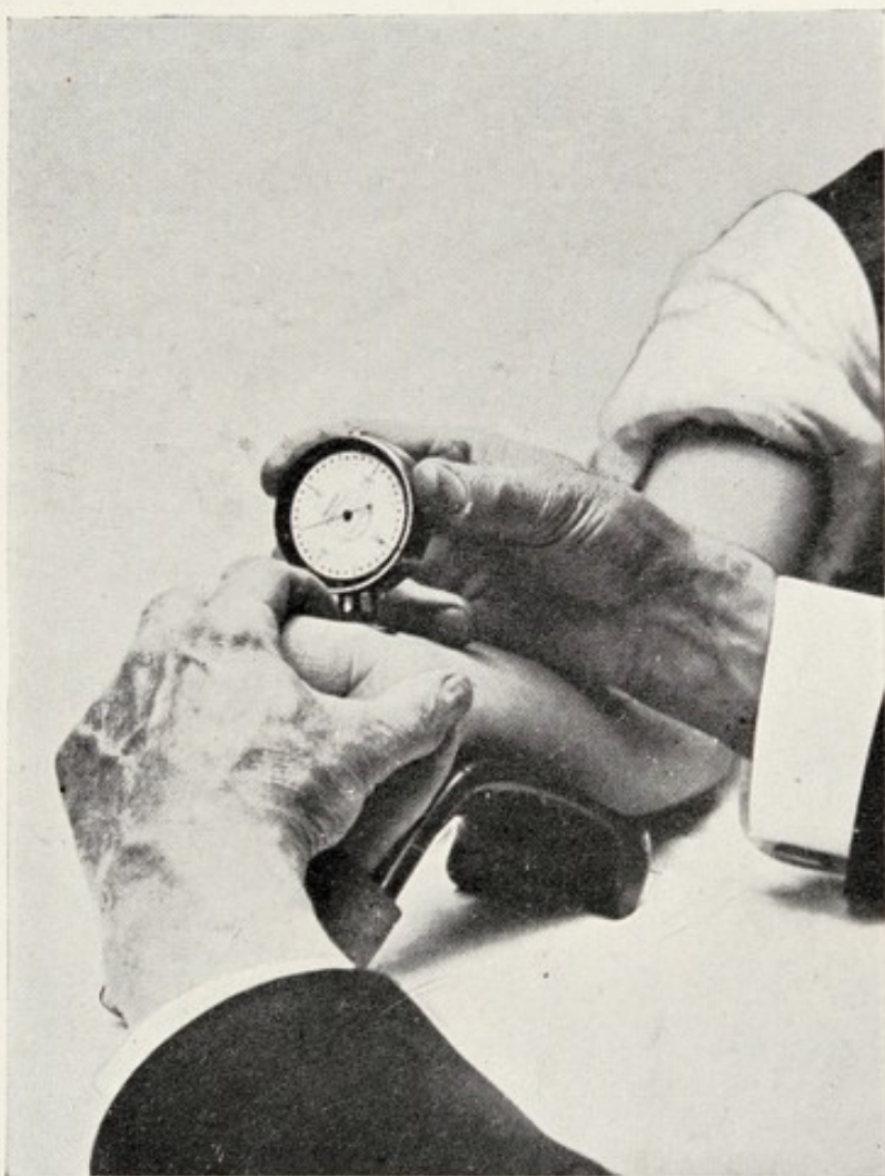
FIG. 7.—MODE OF USING THE ARTERIOMETER, THE WRIST BEING EXTENDED ON A WRIST-REST.
