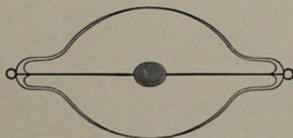
FIG. 36. Tube with continuous metallic conductor. (Rollins.)
