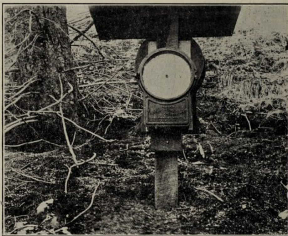
Fig. 8. Instrument shelter, showing thermograph and psychrograph in position.
