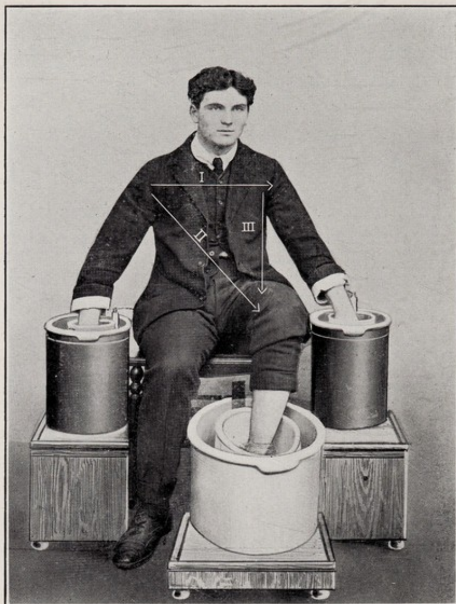
Fig. 4. Photograph of a subject as connected for observation. The two arms and the left leg are used, and curves are taken from the three leads which are represented by the arrows drawn upon the figure. The zinc sulphate is placed in the outer vessels of the electrodes shown in this figure.
