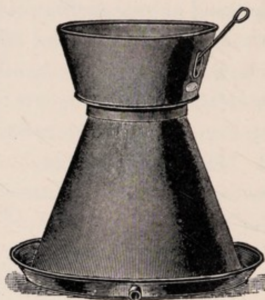
FIG. 52. — Practical milk coolers for farm use. The one on the left is more efficient, but more expensive. Cold water, preferably ice water, is used for cooling.
