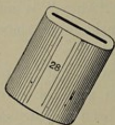
FIG. 44.—Lead Counterweight for Platinum Dish. Made from half-inch lead pipe flattened.
