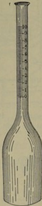
FIG. 37.—Babcock Milk-test Bottle.
