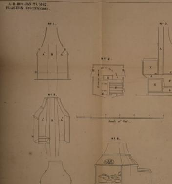
No. 1 Section of hir and Soot flues with damper to regulate the Eurent as they stand over the bear or brens and separate the boilers from the hot plate.
