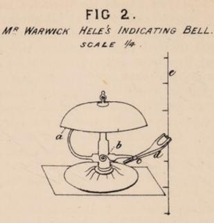
a. Hammer which strikes the bell. b. Spring which keeps hammer nearly in contact with bell. c. Joint. d. Lever which exactly conterbalances spring. e. Strap with projecting pins. (Fig. 1 j. o. h.)
