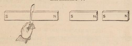
Having proved that the Patented Skeuasma Strip is a perfectly polarised magnet, possessing both an attractive and repellant influence, cut it into two equal parts, when it will be found that each piece has assumed a perfectly polarised condition capable of producing with equal readiness all the experiments made with the strip before division.
