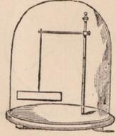
Pass a piece of silk through the centre of the strip, so that when suspended it shall be perfectly level. Cover it with a glass shade to prevent any current of air interfering with its movements, when it will settle down into a north and south position.
