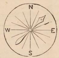
Take a strip of the Skeuasma and gradually present it to the compass. As it approaches, the needle will be deflected; either attracted or repelled. If the north end be repelled it is the north end of the Skeuasma that is presented.
