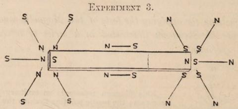
By passing the compass slowly round the Skeuasma strip the needle will assume the different positions indicated in the annexed diagram.
