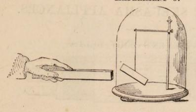
If from the outside is presented another strip of the Skeuasma, the suspended strip will be immediately deflected according to the end presented, precisely in the same manner as the needle of a compass.
