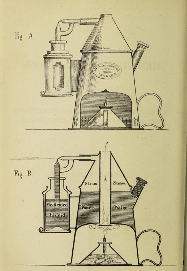
Apparatus for the production of Medicated Vapours.
