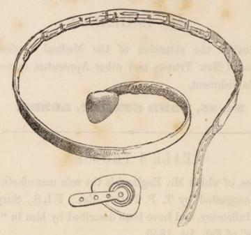
This Truss, like the former, consists of an elastic girdle of steel, and a hard pad of special form, acted upon by a spiral spring.
