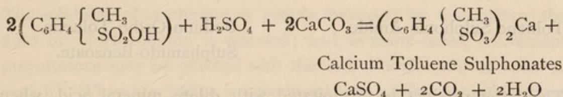
3.—The calcium salts are now treated with carbonate of sodium to obtain the sodium salts with precipitation of carbonate of calcium.
