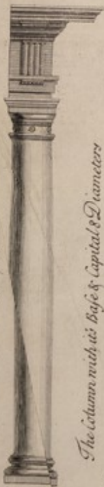
The Column with its Base & Capital 8 Diameters
