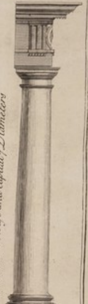
The Column Base and Capital 7 Diameters
