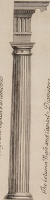
The Column Base and Capital 8 Diameters
