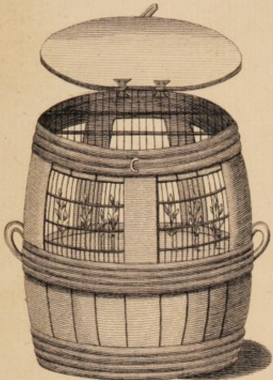
The Cask for sowing East-India seeds with the openings defended by Wire.
