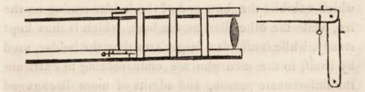
on hinges by drawing out the iron pin, when the weight of the last stave, which is of iron, instantly makes it fall and hang vertically in the water. When this is let down as close as possible to the person in jeopardy, he may, by a very small effort, get his feet on it, and then either K ascend ascend by his own efforts, or greatly facilitate the efforts of another, who may have advanced on the ladders to draw him out.
