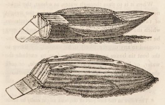
2nd. A Portable gig boat made of wicker for the advantage of extreme lightness.
