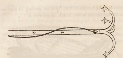
5th. An *Elongatable* grappling rod, which in cases where the body has sunk beneath the ice can be instantly adapted to any common depth of water, for the purpose of grappling for and bringing the sufferer to the surface.
