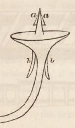
a a are barbs fitting with springs into mortices on the sides of the point.
