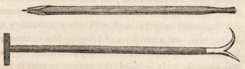
4th. Sprits armed with iron points, which, by sticking in the ice, are used for impelling the boats forward.
