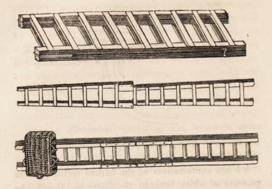
6th. Portable ladders for communicating with the boat from the ice, in cases where the current may have carried the body from the place at which it first sunk. These ladders may be *lengthened* by *unfolding* or *fitting* in, and made *buoyant* as may suit the occasion for which they are intended.
