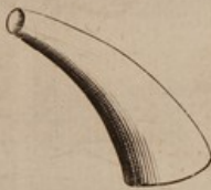
The figure of an Iron retort such as are used at the quicksilver worke at Idria.
