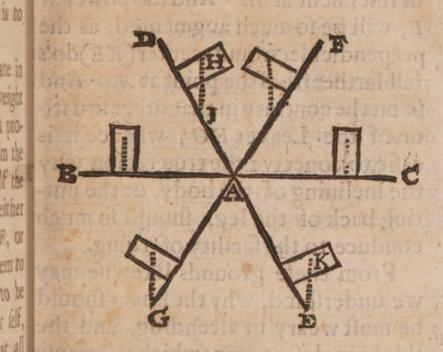
Where A, is supposed to be the place of the prop or fulciment, B C,a Leaver which stands horizontally, the power and the weight belonging unto it, being equal both in themselves, and also in their distances from the prop.
