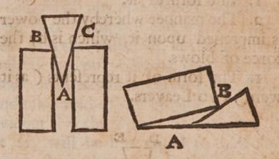
Therefore Ubaldus hath more exactly applied the several parts of it according to this form, that the point A, should be as the common fulciment, in which both the fides do meet, and (as it were) uphold one another; the points B, and C, representing that part of the Leavers where the weight is placed.
