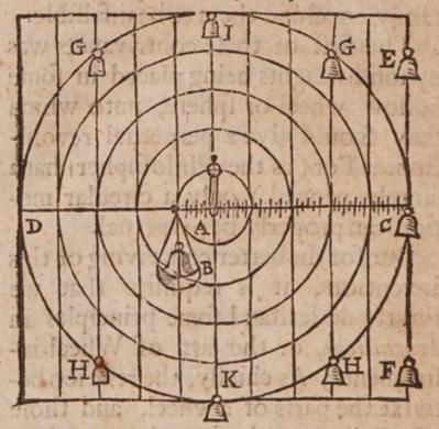
Thus suppose the center to be at A, and the Diameter of the wheel DC, to be divided into equal parts (as is here expressed) it is evident according to the former ground, that one pound at C, will equiponderate to five pound at B, because there is such a proportion betwixt their several distances from the Center. And it is not material whether or no these several weights be placed horizontally; for though B do hang lower than
