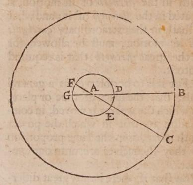
Let the line GAB, represent a ballance or leaver, the weight being supposed at the point G, the sulciment at A, and the power sustaining the weight at B. Suppose the point G, unto which the weight is fastned, to be elevated unto F, and the opposite point B, to be depressed unto C; it is evident that the arch FG, or (which is all one) DE, doth shew the space of the weight, and the arch BC, the motion of the power. Now both
