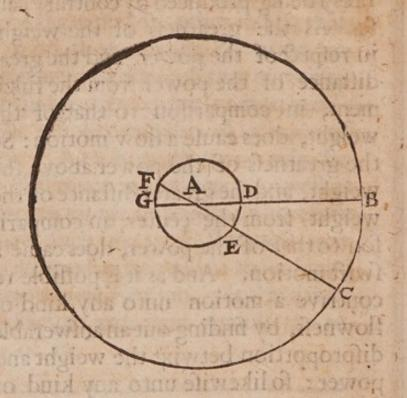
In the Diagram set down before, if we suppose F to be the place of the power, and C of the weight, the point A being the fulciment or center, then in the same space of time, wherein the power does move from F to G, the weight will pass from C to B. These distances having the same disproportion unto one another, as there is betwixt A F, and A C, which is supposed to be quadruple. So that in this example, the weight will move four
