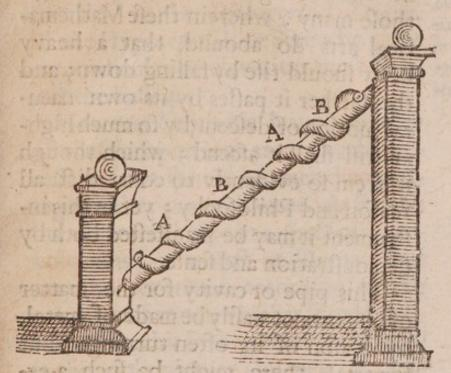
Where you see there is a Cylinder AA, and a spiral cavity or pipe twining about it, according to equal revolutions BB. The axis and centers of its motions are at the points CD, upon which being turned, it will so happen that the same part of the pipe which was now lowermost, will presently become higher, so that the water does ascend by descending; assending in comparison to the whole instrument, and descending in respect
