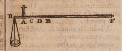
Suppose an equal weight at C, unto that at B, (which points are both equally distant from the center A,) it is evident that then the beam B F, will hang horizontally. But if the weight supposed at C, be unequal to that at B, or if there be an equal weight at D E, or any of the other unequal distances; the Beam must then necessarily decline.
