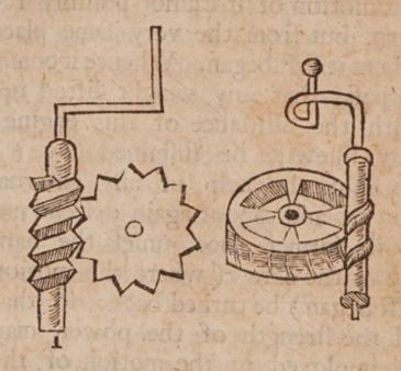
For the composure of which, instead of the female, or concave screw, there must be a little wheel, with some notches in it, equivalent to teeth, by which the other may take hold of it, and turn it round, as in these other figures.
