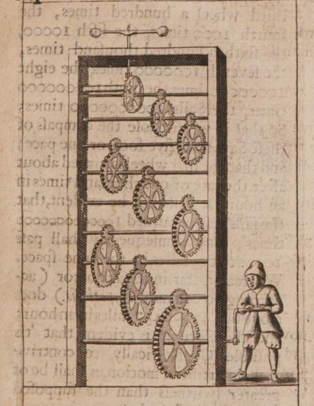
It may then be evident, that one revolution of the first wheel, will turn the nut, and consequently the second wheel on the same axis ten times, the third
