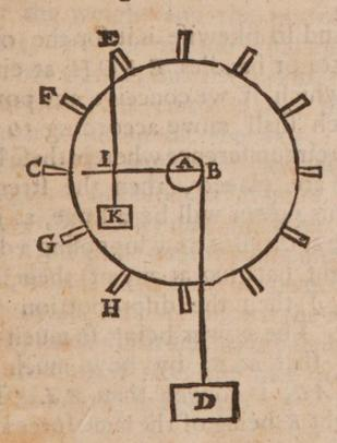
Suppose AB, for the Semidiameter of the Axis or Cylinder, and AC, for the Semidiameter of the rundle, with the spokes; then the power D 4 at
