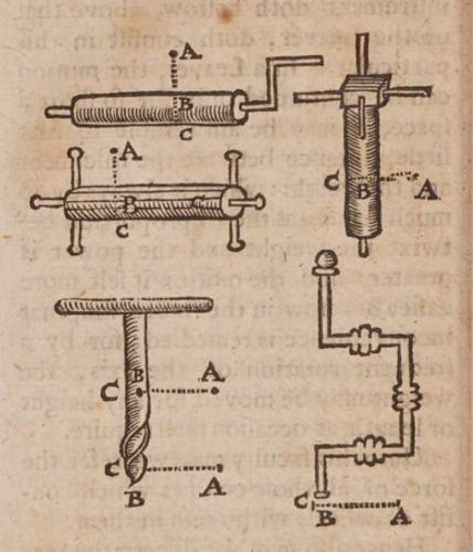
All which are but several kinds of this third Mechanical faculty. In which the points A B C, do represent the places of the power, the fulciment, and the weight. The power being in the same proportion unto the weight, as B C is unto B A.
