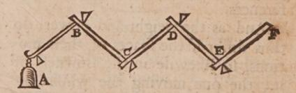
In which, as each instrument doth diminish the weight according to a decuple proportion, so also do they diminish the space and slowness of its motion. For if we should conceive the first Leaver B, to be depressed unto its lowest, suppose ten foot, yet the weight A, would not be raifed
