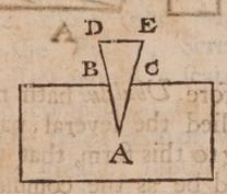
Each fide AD, and AE, being one, the points BC, being instead of several props or fulciments; the weight to be moved, at A, and the power that should move it, being applyed to the top DE, by the force of Mechan. some stroak or blow, as Aristotle c. 8. hath explained the several parts of this faculty. But now, because this instrument may be so used that the E3 point
