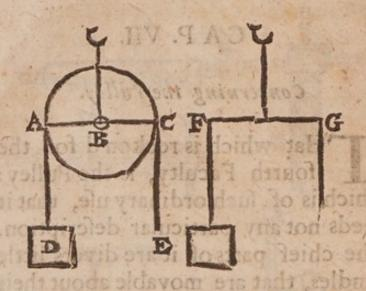
The Diameter AC, being as the beam of a ballance, of which B is the prop or center. Now the parts A, and C, being equally distant from this center, therefore the power at E, must be equal to the weight at D, it being all one as if the power and the weight were fashed by two several strings at the ends of the ballance F G.
