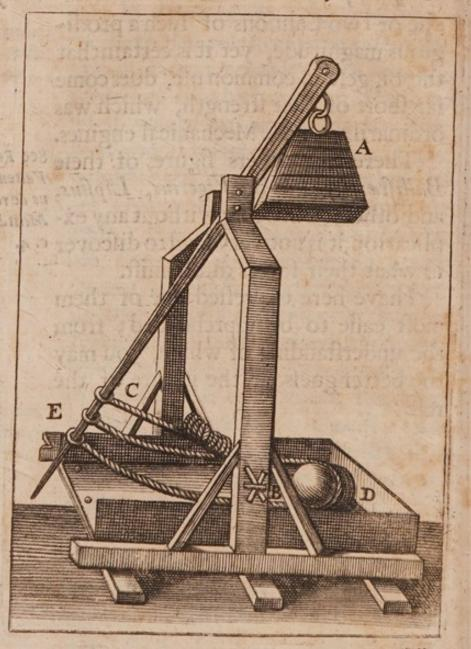
That great box or cavity at A, is supposed to be full of some heavy weight, and is forced up by the turning
