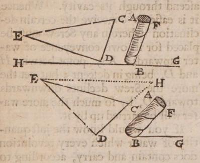
then the inclination of the revolutions in it, will be increased by the angle EDH, though these revolutions will still remain in a kind of ascent, so that water cannot be turned through them.
