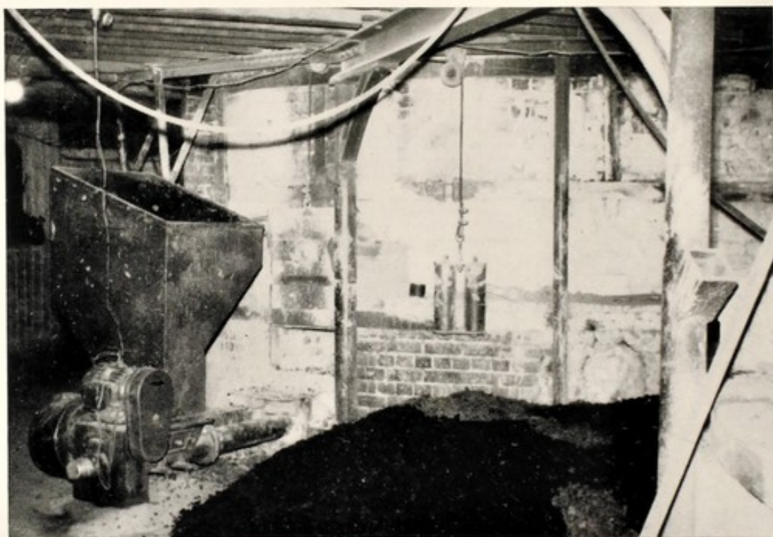
Tile kiln converted to mechanical stoking
