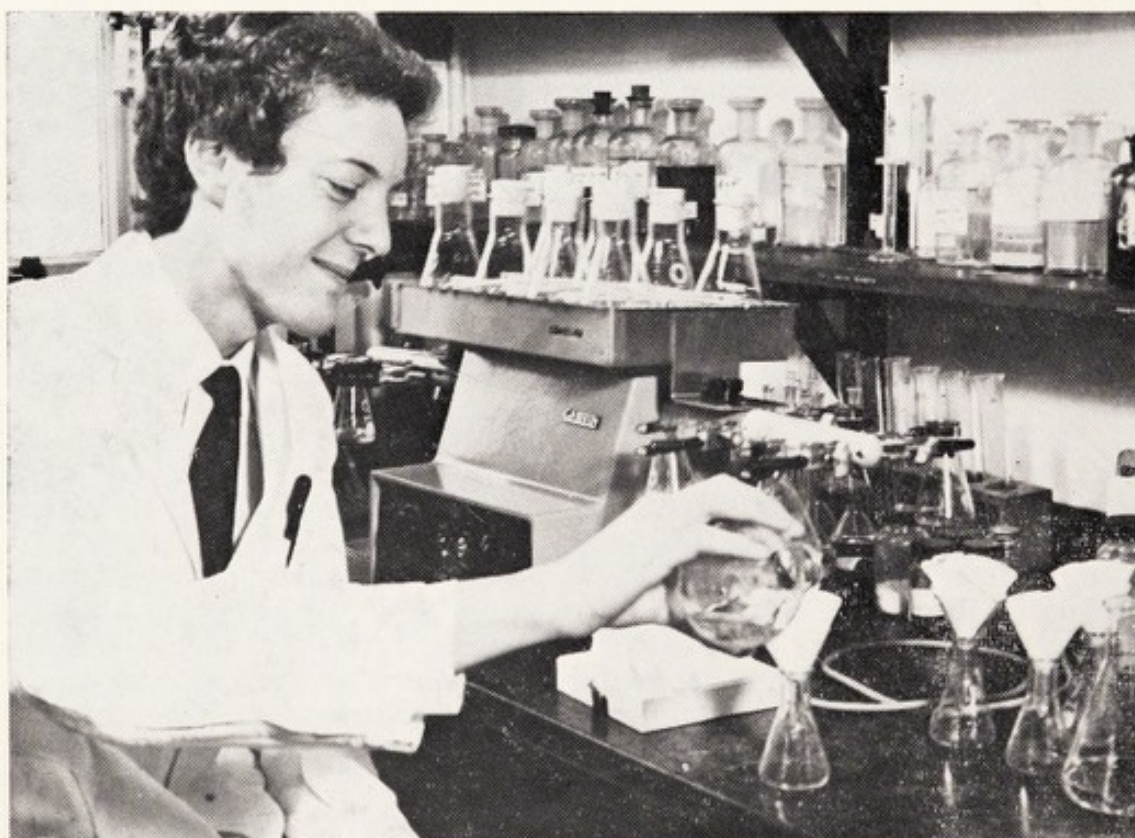
Colorimetric determination of sulphate in test boreholes associated with new trunk sewer
