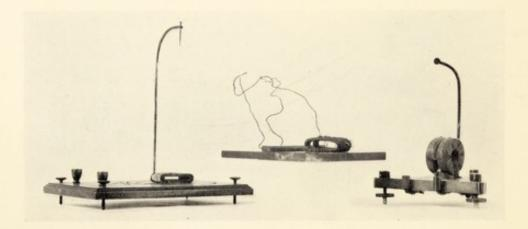
Early galvanometers made and used by Faraday
