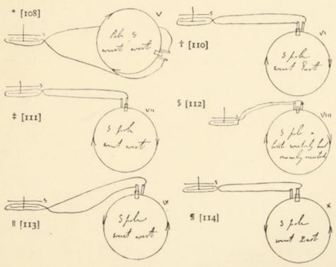
115. Hence changing the direction of the motion of the plate changes the current, and also changing the conductors to the right or left reverses the current.
